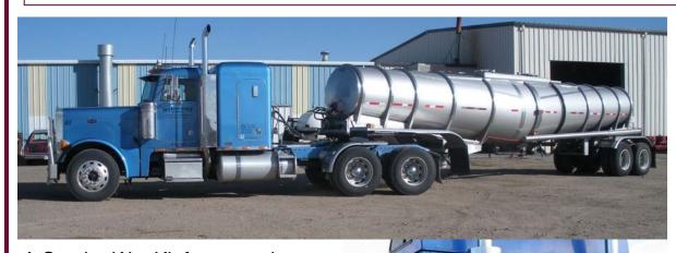
A Combo Wet Kit for operating multiple types of trailers. With a 50 gallon reservoir you can handle end-dumps, and with high and low pressure, you can pull most kinds of belt, chain, shuffle-floor, tanker and implement trailers.
