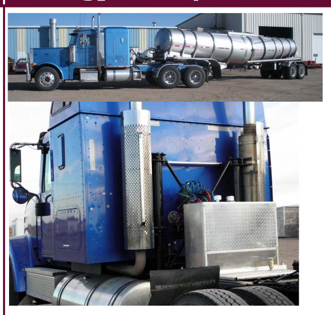
Suitable for Tanker applications with a drive-line between the truck and trailer. The hydraulic valve and motor is mounted on the truck. We have other kits available with higher flow and pressure.
